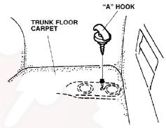
Using a utility knife, cut the carpet around each hook. Make your cut as close to the hook as possible. Remove and discard the cut piece of carpet, and remove the hooks.
