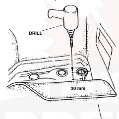
Lift up the corner of the carpet, and locate the hole you just drilled. With your finger on the carpet and over the hole, lay the carpet back to its original position. Using an awl, poke the floor carpet to locate the hole. Repeat on the other side of the trunk floor.
