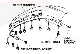
7. Install a self-tapping screw through each spring nut.
