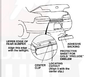
Hold the emblem firmly against the rear bumper with the palm of your hand, while you remove the protective sheet.
