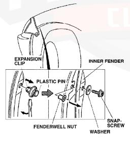
8. Pull the side mask back toward the wheelwell, smooth out any wrinkles, and then snap the mask onto the snap-screw. Do this for both sides.
