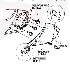
• Remove the three self-tapping screws from around the speaker.
