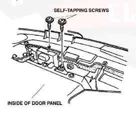
Inside the door panel, press the retaining tab with a flat-tip screwdriver, and raise the remote control door mirror switch.
