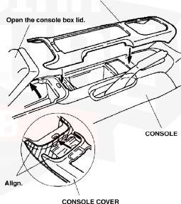
12. Thoroughly clean the bonding surfaces where the console cover will attach; remove the adhesive backing from the console cover, and attach the cover to the console by pressing firmly with the palms of both hands. Remove the masking tape.
