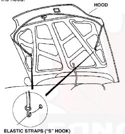
Secure the mask by hooking the two elastic straps to the holes in the back of the hood.
