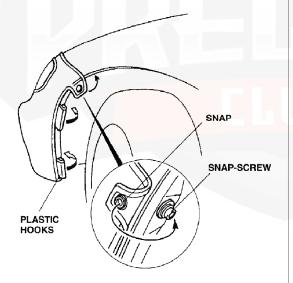
12. Pull the mask back toward the wheelwell, smooth out any wrinkles, and hook the plastic hooks around the edge of the fender. Repeat on the other side of the vehicle. 13. Put these instructions and the expansion clips removed in step 5 into the storage bag, and place it in the trunk for future use.
