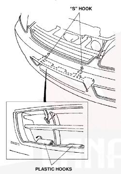
11. Snap the nose mask to the snap-screw. Repeat on the other side of the vehicle.
