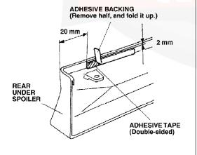
Insert the four retaining plates of the rear under spoiler into the slits in the bottom of the rear bumper, and reinstall the three bolts removed in step 2. Do not tighten the bolts yet.
