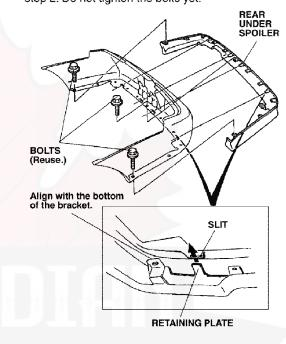
Install the six bumper bolts from the kit and two of the clips removed in step 2. (The remaining six clips removed in step 2 are not reused.)
