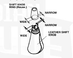
Thread the new leather shift knob onto the shift lever until it is tight. Turn the knob clockwise until the shift pattern on top is in the proper direction.
