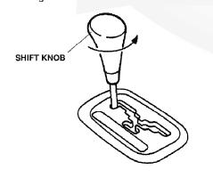
Remove the shift knob ring from the shift knob by pulling it up and rocking it back and forth.
