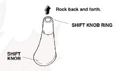
Slide the shift knob ring onto the new leather shift knob by aligning the ring and the knob.
