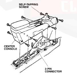
Turn over the center console, and remove the four self-tapping screws fastening the boot. Install the boot from the kit. Note the installation direction.
