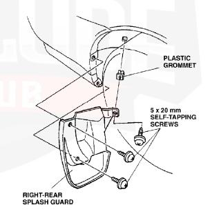
Position the right-rear splash guard on the rear bumper, and install three of the 5 x 20 mm self-tapping screws supplied.
