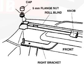
10. Install the two caps over the 5 mm flange nuts.
