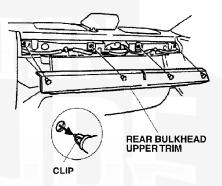
2. Pry up on the four retaining clips, and remove the rear speaker grille.
