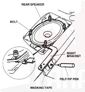
Lightly center-punch the mark and remove the masking tape. While wearing eye protection, drill a 6 mm hole through the body.
