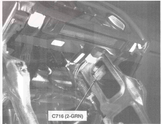
77. Center of Dash (Panel Removed)
