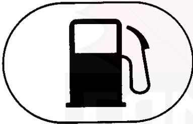
LOW FUEL INDICATOR LIGHT (In the sub gauge assembly)
